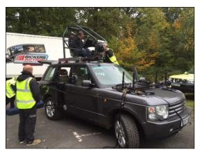
All the controls of the vehicle are relocated into a driver capsule secured to the roof of the car. The engineering behind this Rig is that all controls are relocated to the roof of the car – steering, brakes, throttle and gear control which must always be an Automatic Transmission car. No manufacturer's control systems are modified just relocated. The aesthetics / Interior of the Pod vehicle is only changed by the fact the car is fitted with a very large roof rack.
