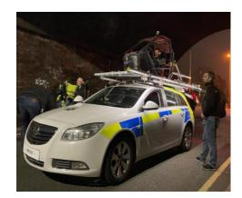
All the controls of the vehicle are relocated into a driver capsule secured to the roof of the car. The engineering behind this Rig is that all controls are relocated to the roof of the car – steering, brakes, throttle and gear control which must always be an Automatic Transmission car. No manufacturer's control systems are modified just relocated. The aesthetics / Interior of the Pod vehicle is only changed by the fact the car is fitted with a large roof rack.
